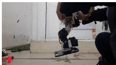
Gambar 11 Walking Trajectory Kaki Kanan (Tampak Samping)
